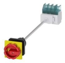
SENTRON, Switch disconnector 3LD, emergency switching-off switch, 4-pole, Iu: 32 A, operating power / at AC-23 A 400 V: 11.5 kW, floor mounting with door coupling, rotary operating mechanism, Red / yellow, central mounting 22.5 mm of the handle
