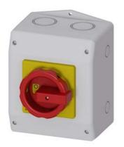
SENTRON, Switch disconnector 3LD, emergency switching-off switch, 6-pole, lu: 25 A, operating power / at AC-23 A 400 V: 9.5 kW, Molded plastic encapsulation for metric cable gland, rotary operating mechanism, red/yellow
