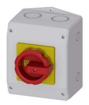
SENTRON, Switch disconnector 3LD, emergency switching-off switch, 6-pole, Iu: 25 A, operating power / at AC-23 A 400 V: 9.5 kW, Molded plastic encapsulation for metric cable gland, 1 NC, 1 NO, rotary operating mechanism, red/yellow
