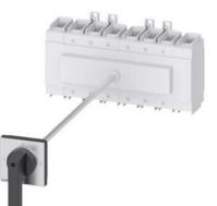
SENTRON, switch disconnector 3LD, change-over switch, 4-pole, lu: 160 A, operating performance / at AC-23 A at 400 V: 75 kW, floor mounting with door coupling, knob-operated mechanism, black, 4-hole mounting of the handle
