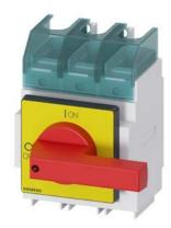
SENTRON, switch disconnector 3LD, emergency switching-off switch, 3pole, lu: 160 A, operating performance / at AC-23 A at 400 V: 75 kW, installation in distribution boards, knob-operated mechanism, red/yellow, handle direct at the switch
