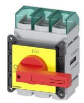
SENTRON, Switch disconnector 3LD, emergency switching-off switch, 3-pole, Iu=250 A, operating power / at AC-23 A 400 V: 132 kW, front-mounted, knob-operated mechanism, red/yellow, 4-hole mounting of the handle
