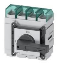
SENTRON, Switch disconnector 3LD, main switch, 4-pole, lu=250 A, Operating power / at AC-23 A at 400 V: 132 kW, front-mounted, knob-operated mechanism, black, 4-hole mounting of the handle
