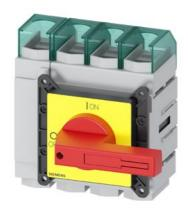
SENTRON, Switch disconnector 3LD, emergency switching-off switch, 4-pole, lu=250 A, operating power / at AC-23 A 400 V: 132 kW, front-mounted, knob-operated mechanism, red/yellow, 4-hole mounting of the handle
