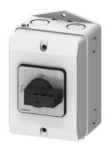
SENTRON switch disconnector 3LD in molded-plastic enclosure , repair and maintenance switch with EMC plate, 3-pole lu: 25A, AC23A 400V at 50/60Hz: 9,5kW, used with frequency converter: AC20 400V at 0-550Hz: 5,5kW, 1NO + 1NC 20-150ms leading, molded-plastic encapsulation for metric cable gland, knob-operated mechanism, black, lockable in 0- and I-position, incl. cable shield clamps
