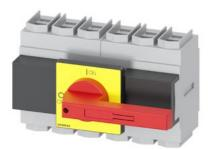
SENTRON, Switch disconnector 3LD, emergency switching-off switch, 6-pole, Iu=250 A, operating power / at AC-23 A 400 V: 132 kW, front-mounted, knob-operated mechanism, red/yellow, 4-hole mounting of the handle
