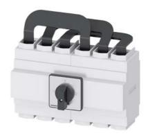
SENTRON, Switch disconnector 3LD, change-over switch, 3-pole, lu = 250 A, Operating power / at AC-23 A at 400 V: 132 kW, front-mounted, knoboperated mechanism, black, 4-hole mounting of the handle
