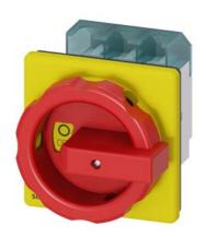
SENTRON, Switch disconnector 3LD, emergency switching-off switch, 3-pole, lu: 63 A, operating power / at AC-23 A 400 V: 22 kW, front-mounted, rotary operating mechanism, Red / yellow, 4-hole mounting of the handle
