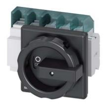
SENTRON, Switch disconnector 3LD, main switch, 4-pole, lu: 63 A, Operating power / at AC-23 A at 400 V: 22 kW, front-mounted, 1 NC, 1 NO, rotary operating mechanism, black, 4-hole mounting of the handle
