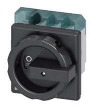
SENTRON, Switch disconnector 3LD, main switch, 4-pole, lu: 63 A, Operating power / at AC-23 A at 400 V: 22 kW, front-mounted, rotary operating mechanism, black, 4-hole mounting of the handle
