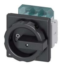
SENTRON, Switch disconnector 3LD, main switch, 3-pole, lu: 63 A, Operating power / at AC-23 A at 400 V: 22 kW, front-mounted, 1 NC, 1 NO, rotary operating mechanism, black, 4-hole mounting of the handle
