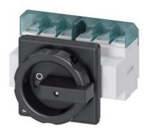
SENTRON, Switch disconnector 3LD, main switch, 6-pole, lu: 63 A, Operating power / at AC-23 A at 400 V: 22 kW, front-mounted, rotary operating mechanism, black, 4-hole mounting of the handle
