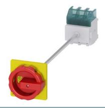
SENTRON, Switch disconnector 3LD, emergency switching-off switch, 3-pole, Iu: 63 A, operating power / at AC-23 A 400 V: 22 kW, floor mounting with door coupling, rotary operating mechanism, Red / yellow, 4-hole mounting of the handle
