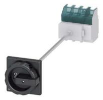
SENTRON, Switch disconnector 3LD, main switch, 4-pole, lu: 63 A, Operating power / at AC-23 A at 400 V: 22 kW, floor mounting with door coupling, rotary operating mechanism, black, 4-hole mounting of the handle
