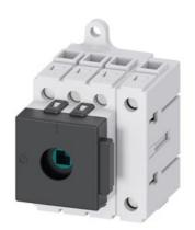
Load disconnector 3LD3, lu 25 A Main switch 3-pole + N Rated operating capacity at AC-23 A at 400V 9.0kW Installation in distribution boards, Basic switch without Knob-operated mechanism
