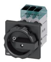
Load disconnector 3LD3, lu 32 A Main switch 3-pole Rated operating capacity for AC-23 A at 400V 11.5kW Front plate mounting Basic switch with Central hole mounting 22.5mm Rotating drive black 66 x 66 mm
