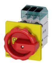
Load disconnector 3LD3, lu 32 A Main switch 3-pole Rated operating capacity for AC-23 A at 400V 11.5kW Front plate mounting Basic switch with Central hole mounting 22.5mm Rotary actuator red / yellow 66 x 66 mm
