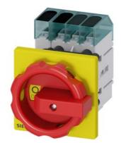
Load disconnector 3LD3, lu 32 A Main switch 3-pole + N Rated operating capacity for AC-23 A at 400V 11.5kW Front plate mounting Basic switch with Central hole mounting 22.5mm Rotary actuator red / yellow 66 x 66 mm
