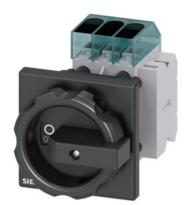
Load disconnector 3LD3, lu 32 A Main switch 3-pole Rated operating capacity for AC-23 A at 400V 11.5kW Front plate mounting Basic switch with Central hole mounting 22.5mm Rotating drive black 66 x 66 mm with auxiliary switch 10E + 1S
