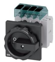
Load disconnector 3LD3, lu 32 A Main switch 3-pole + N Rated operating capacity for AC-23 A at 400V 11.5kW Front plate mounting Basic switch with Central hole mounting 22.5mm Rotating drive black 66 x 66 mm with auxiliary switch 10E + 1S
