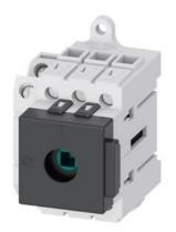
Load disconnector 3LD3, lu 25 A Main switch 3-pole Rated operating capacity at AC-23 A at 400V 9.0kW Installation in distribution boards, Basic switch without Knob-operated mechanism with auxiliary switch 1OE + 1S
