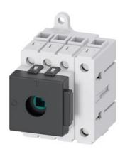
Load disconnector 3LD3, lu 40 A Main switch 3-pole + N Rated operating capacity at AC-23 A at 400 V 18.5 kW Installation in distribution boards, Basic switch without Knob-operated mechanism
