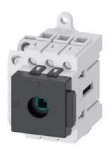
Load disconnector 3LD3, lu 40 A Main switch 3-pole Rated operating capacity at AC-23 A at 400 V 18.5 kW Installation in distribution boards, Basic switch without Knob-operated mechanism with auxiliary switch 1OE + 1S
