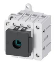
Load disconnector 3LD3, lu 40 A Main switch 3-pole + N Rated operating capacity at AC-23 A at 400 V 18.5 kW Installation in distribution boards, Basic switch without Knob-operated mechanism with auxiliary switch 1OE + 1S
