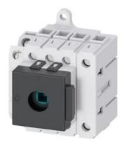
Load disconnector 3LD3, lu 25 A Main switch 3-pole + N Rated operating capacity at AC-23 A at 400V 9.0kW Installation in distribution boards, Basic switch without Knob-operated mechanism with auxiliary switch 1OE + 1S
