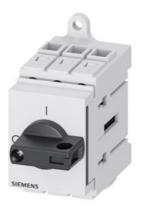
Load disconnector 3LD3, lu 25 A Main switch 3-pole Rated operating capacity at AC-23 A at 400V 9.0kW Installation in distribution boards, Basic switch with selector knob black
