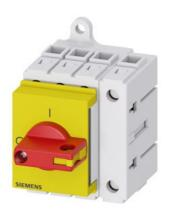
Load disconnector 3LD3, lu 25 A Main switch 3-pole + N Rated operating capacity at AC-23 A at 400V 9.0kW Installation in distribution boards, Basic switch with selector knob red / yellow
