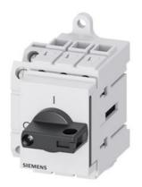
Load disconnector 3LD3, lu 25 A Main switch 3-pole Rated operating capacity at AC-23 A at 400V 9.0kW Installation in distribution boards, Basic switch with selector knob black with auxiliary switch 1OE + 1S
