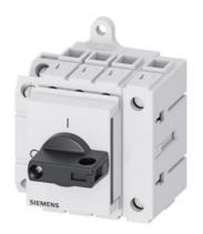
Load disconnector 3LD3, lu 25 A Main switch 3-pole + N Rated operating capacity at AC-23 A at 400V 9.0kW Installation in distribution boards, Basic switch with selector knob black with auxiliary switch 1OE + 1S
