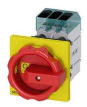
Load disconnector 3LD3, lu 16 A Main switch 3-pole Rated operating capacity at AC-23 A at 400V 7.5kW Front plate mounting Basic switch with Central hole mounting 22.5mm Rotary actuator red / yellow 66 x 66 mm
