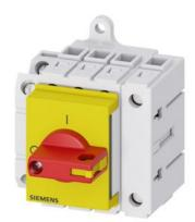
Load disconnector 3LD3, lu 25 A Main switch 3-pole + N Rated operating capacity at AC-23 A at 400V 9.0kW Installation in distribution boards, Basic switch with selector knob red / yellow with auxiliary switch 1OE + 1S
