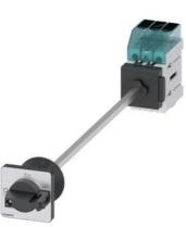
Load disconnector 3LD3, lu 25 A Main switch 3-pole Rated operating capacity at AC-23 A at 400V 9.0kW floor mounting Basic switch with door coupling Central hole mounting 22.5mm Toggle drive black 48x48 mm
