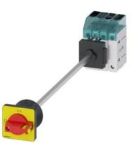
Load disconnector 3LD3, lu 25 A Main switch 3-pole + N Rated operating capacity at AC-23 A at 400V 9.0kW floor mounting Basic switch with door coupling Central hole mounting 22.5mm Toggle drive red / yellow 48x48 mm
