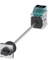
Load disconnector 3LD3, lu 25 A Main switch 3-pole Rated operating capacity at AC-23 A at 400V 9.0kW floor mounting Basic switch with door coupling Central hole mounting 22.5mm Toggle drive black 48x48 mm with auxiliary switch 10E + 1S
