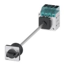
Load disconnector 3LD3, lu 25 A Main switch 3-pole + N Rated operating capacity at AC-23 A at 400V 9.0kW floor mounting Basic switch with door coupling Central hole mounting 22.5mm Toggle drive black 48x48 mm with auxiliary switch 1OE + 1S
