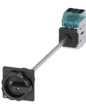
Load disconnector 3LD3, lu 25 A Main switch 3-pole Rated operating capacity at AC-23 A at 400V 9.0kW floor mounting Basic switch with door coupling Central hole mounting 22.5mm Rotating drive black 66 x 66 mm
