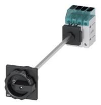
Load disconnector 3LD3, Iu 25 A Main switch 3-pole + N Rated operating capacity at AC-23 A at 400V 9.0kW floor mounting Basic switch with door coupling Central hole mounting 22.5mm Rotating drive black 66 x 66 mm
