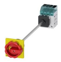
Load disconnector 3LD3, lu 25 A Main switch 3-pole + N Rated operating capacity at AC-23 A at 400V 9.0kW floor mounting Basic switch with door coupling Central hole mounting 22.5mm Rotary actuator red / yellow 66 x 66 mm
