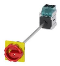
Load disconnector 3LD3, lu 25 A Main switch 3-pole Rated operating capacity at AC-23 A at 400V 9.0kW floor mounting Basic switch with door coupling Central hole mounting 22.5mm Rotary actuator red / yellow 66 x 66 mm with auxiliary switch 10E + 1S
