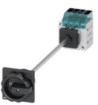
Load disconnector 3LD3, lu 25 A Main switch 3-pole + N Rated operating capacity at AC-23 A at 400V 9.0kW floor mounting Basic switch with door coupling Central hole mounting 22.5mm Rotating drive black 66 x 66 mm with auxiliary switch 1OE + 1S
