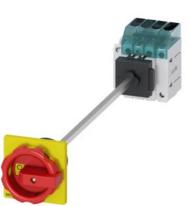
Load disconnector 3LD3, lu 25 A Main switch 3-pole + N Rated operating capacity at AC-23 A at 400V 9.0kW floor mounting Basic switch with door coupling Central hole mounting 22.5mm Rotary actuator red / yellow 66 x 66 mm with auxiliary switch 10E + 1S
