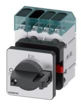
Load disconnector 3LD3, lu 25 A Main switch 3-pole + N Rated operating capacity at AC-23 A at 400V 9.0kW Front plate mounting Basic switch with Central hole mounting 22.5mm Toggle drive black 48x48 mm
