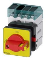
Load disconnector 3LD3, lu 25 A Main switch 3-pole + N Rated operating capacity at AC-23 A at 400V 9.0kW Front plate mounting Basic switch with Central hole mounting 22.5mm Toggle drive red / yellow 48x48 mm
