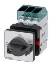
Load disconnector 3LD3, lu 25 A Main switch 3-pole Rated operating capacity at AC-23 A at 400V 9.0kW Front plate mounting Basic switch with Central hole mounting 22.5mm Toggle drive black 48x48 mm
