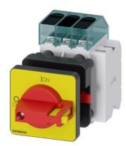
Load disconnector 3LD3, lu 25 A Main switch 3-pole Rated operating capacity at AC-23 A at 400V 9.0kW Front plate mounting Basic switch with Central hole mounting 22.5mm Toggle drive red / yellow 48x48 mm with auxiliary switch 10E + 1S
