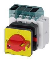
Load disconnector 3LD3, lu 25 A Main switch 3-pole + N Rated operating capacity at AC-23 A at 400V 9.0kW Front plate mounting Basic switch with Central hole mounting 22.5mm Toggle drive red / yellow 48x48 mm with auxiliary switch 1OE + 1S
